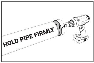
\* Failure to keep the pipe held firmly may result in a defective bevel
